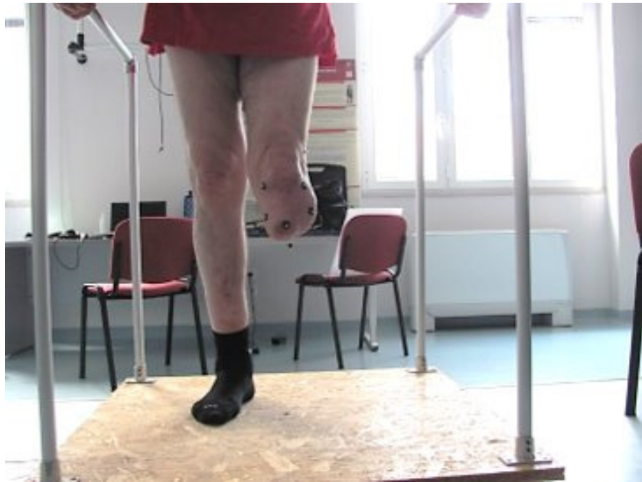
Figure 3. Subject with left transtibial amputation standing upright on the rotating platform with markers placed on his residual limb.
