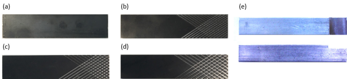
Fig. 1. (a) Flat surface, (b) knurling type “1”, (c) knurling type “2”, (d) knurling type “3” and (e) aluminum specimen
