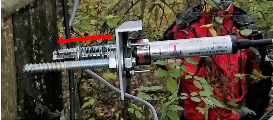
Figure 2: dendrometer installed on a tree. The potentiometer is fixed with two screws that sink into the deepest part of the trunk (not subject to movements), while the tip grazes the bark, and is pushed back and forth by the growth of the plant's radius, as well as from swelling and shrinkage due to daily cycles of hydration and dehydration
