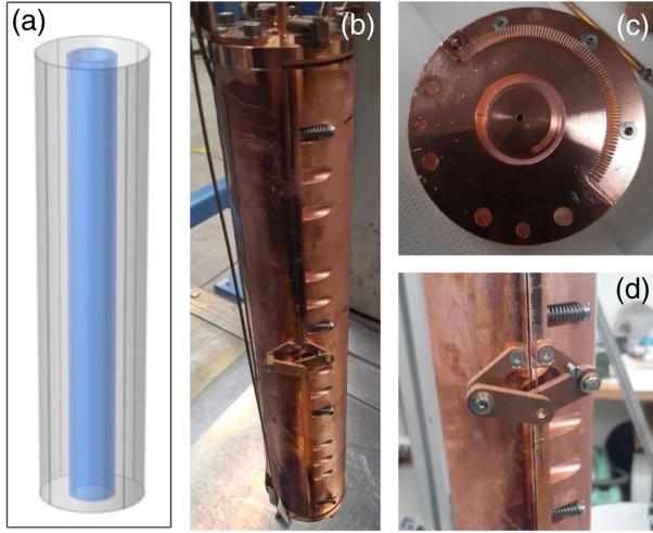
FIG. 1. (a) The microwave resonator is a dielectrically loaded cylindrical cavity. The main structure is a copper cylinder with length 414.3 mm and 60.5 mm diameter (gray area). The cylinder is longitudinally cut in two halves and can be opened with a clamshell-like movement for tuning. It includes a 420 mm long sapphire tube with 21.8 mm inner diameter and 30.2 mm outer diameter (blue area). The sapphire cylinder extends into the cavity end caps by 5.3 mm deep annular grooves. (b) A picture of the cavity mounted in the dilution refrigerator is also shown. (c) End cap with annular grooves for holding the sapphire and springs for keeping the rf contact while tuning. (d) Pantograph for tuning.
