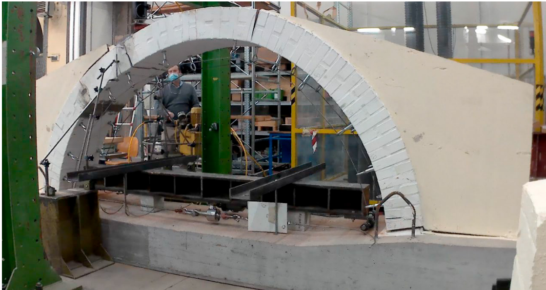
Fig. 4. Deformed shape of the strengthened arch at the last load cycle.
