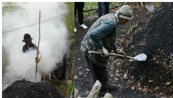
Figure 4. Carbonization process monitoring by the operator: on the left, the operator controls the ignition of the charcoal pile; on the right, the operator covers the base of the charcoal pile with earth to prevent air entrance.
