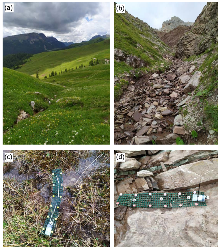
Figure 2.1: Sensors placed along the tributaries of the Rio Valfredda. Left: picture of Zone 1 (a) and a sensor on the grass (c). Right: picture of Zone 2 (b) and a sensor screwed on a rock (d).
