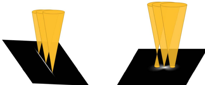
Figure 3.3: Effect of selecting the best focal plane orthogonal to the chief ray for a LGS re-imaging system.
