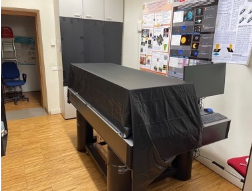
Figure 6.29: The I-WFS test bench with a black cover used to mitigate the effects of stray light.
