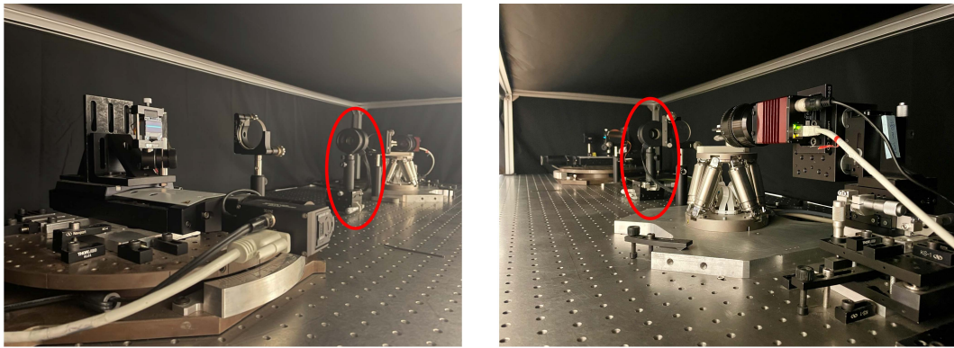
Figure 6.30: View of the I-WFS test bench, equipped with a Deformable Lens conjugated to the pupil plane
