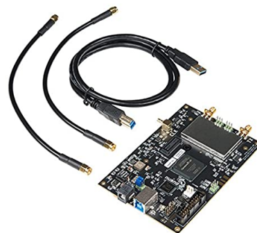
FIGURE 3.5: Nuand BladeRF x40 Rev. 2.
