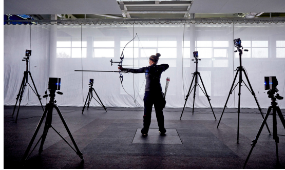
Figure 1.7. Motion Capture Systems are typically composed by several cameras to resolve occlusion problems ( https://www.vicon.com ).
