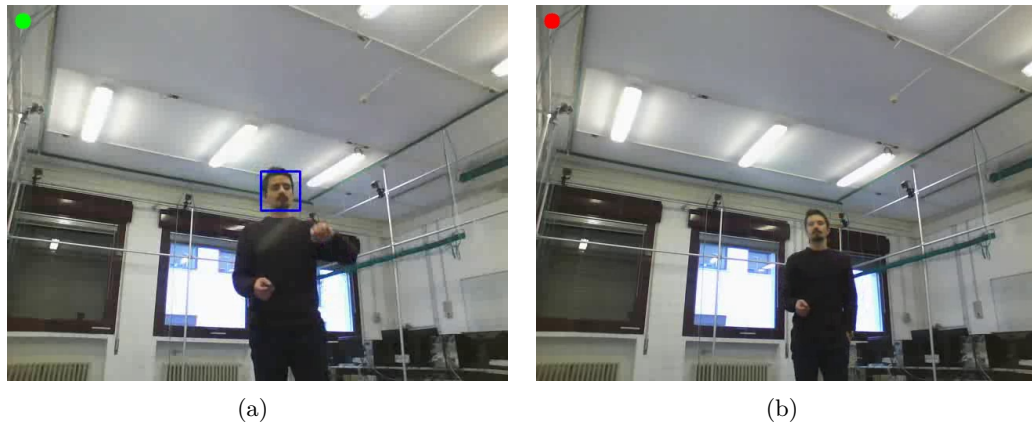
Figure 6.7. Experimental results. a) True Positive example: the target is detected and the camera is active (green marker on left top). b) True Negative example: the target is not detected and the camera is left silent (red marker on left top).
