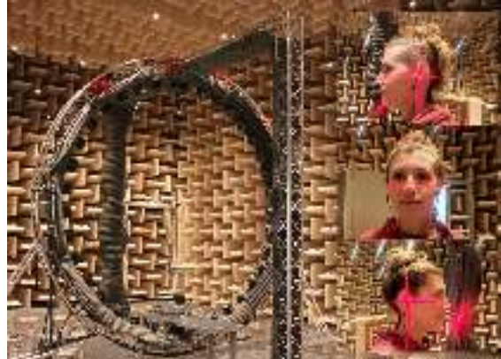
Fig. 5.12 HRIR measurement system at Technical University of Berlin with details of the position procedure using cross line lasers. During the measurement, the subjects is wearing in ear microphones and is sitting on the chair in the center of the loudspeaker array and is continuously rotated to measure a full spherical HRIR data set. In addition, the wire frames on the floor are covered with absorbing material (CC-BY, Fabian Brinkmann).
