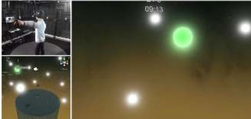
Fig. 4.8: Example active HRTF learning training game. Training setup: (top-left) participant in the experiment room, (bottom-left) third person view of the training platform, (right) participant viewpoint during the training (from [77].)
