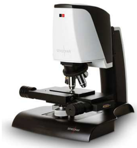
Figure 7.1: Sensofar Plu Neox 3D optical profiler used during surface inspection.
