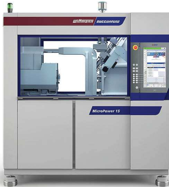
Figure 6.1: Micro injection molding machined utilized through the experimental campaign.
