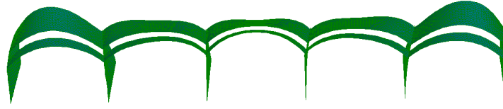
Figure 4.32 First principal modes (3.989Hz and 6.011Hz) calculated by means of the calibrated FE model before the demolition of three spans.
