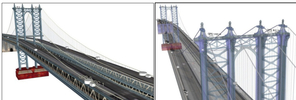
Figure 4.105 Installation of the sensors on the deck and on the Manhattan Tower.
