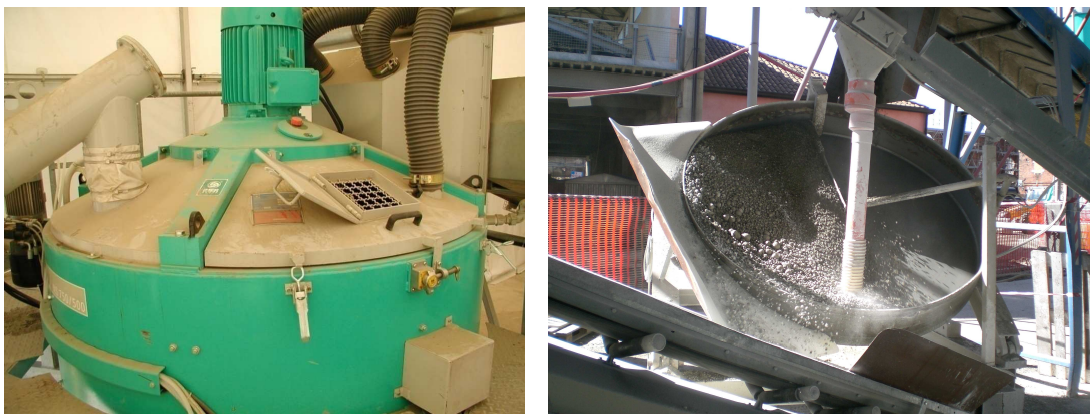
Figure 7.2 - An industrial intensive mixer (left) for blending the initial components and an inclined rotating plate (right, diameter ~ 3 m) for the production of HPSS granular material.
