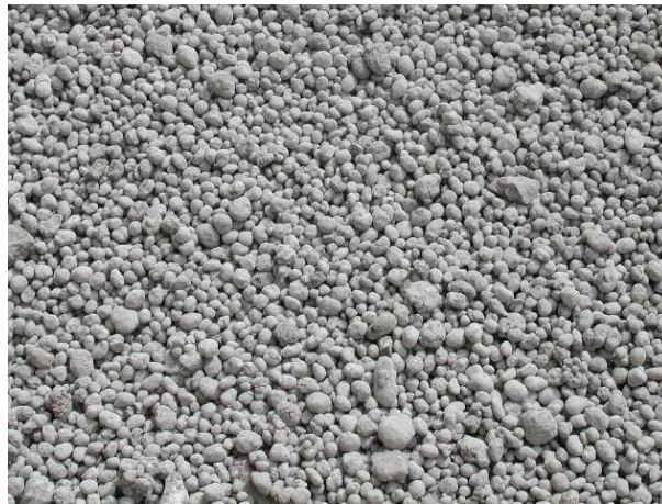
Figure 7.3 - Artificial granular material obtained following the HPSS process. The diameter of the grains ranges approximately from 4 to 16 mm.
