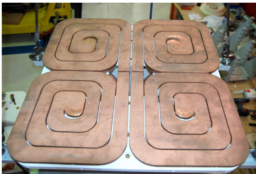
fig. 5.22: Bottom inductor used both to heat and and cool the system.
