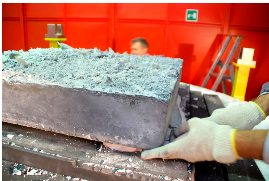
fig. 5.26: A photo from the first ingot extraction step.
