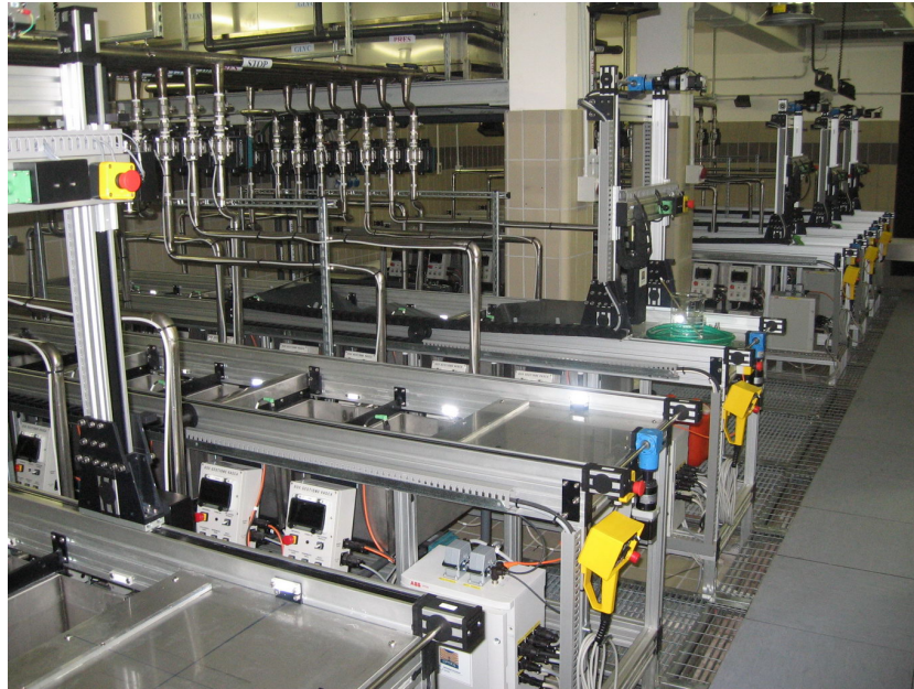
Figure 3.1: The development room in Lab1 at LNGS. The six development lines are visible together with the set of distribution pipes.
