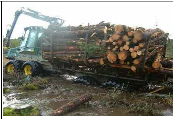
Figure 1.2.b: Forwarder (with 8 t load) operating on a waterlogged site with a shallow (<700 mm depth) solid foundation. The machine caused severe rutting as it sank right down to the underlying solid stratum. This is also a risky situation for working people.
