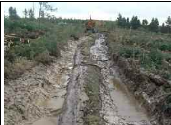
Figure 1.2.a: rutting after 10 passes of a wheeled forwarder (with 8 t load) along a main extraction trail comprising a shallow gley soil overlying solid foundation
