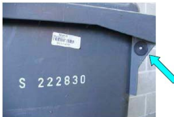
Figure B.5. The transponder for the identification of the residual waste production
