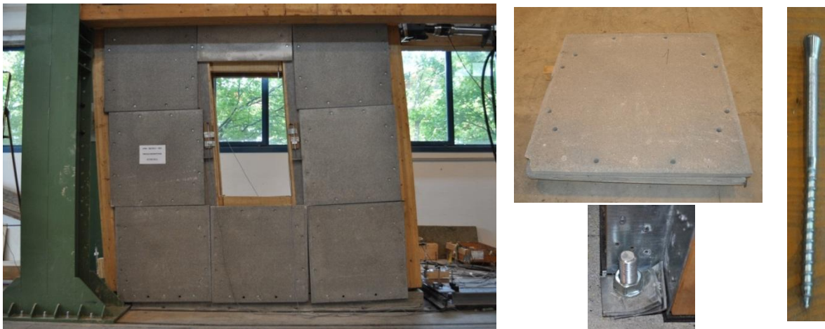
Fig. 7.8 - “Wall C”- configuration at the end of the monotonic ramp test and failure details.
