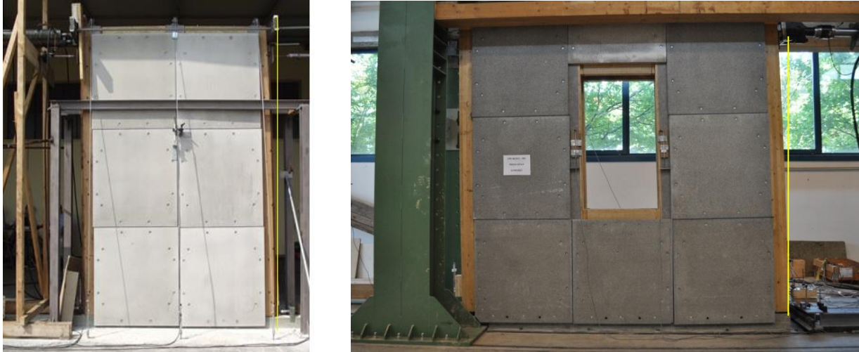
Fig. 7.7 - Wall configuration at the end of the cyclic test - “Wall B” (left) and “Wall C” (right)
