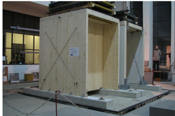
Pseudo-dynamic tests on a 1-storey 3-D specimen [5.13]
