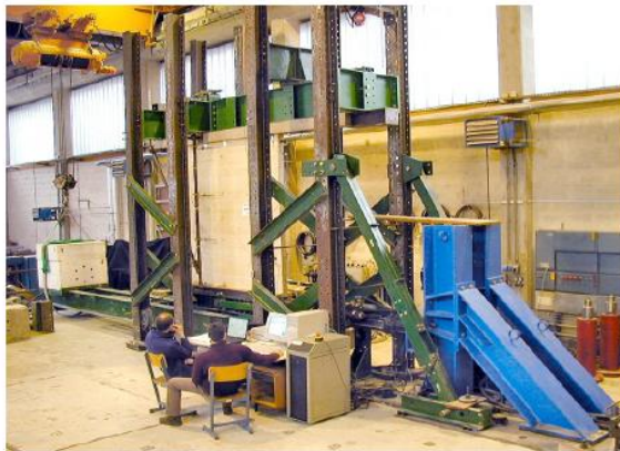
Cyclic test on single wall elements [5.12]
