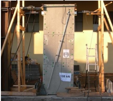
Modular panel braced by screwed RC slabs
