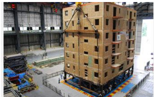
Fig. 6.13 - Building plan (left) and view of the shaken table test (right) [6.6]
