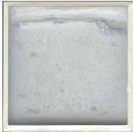
Figure 2.5.: Continuous 4 mm \text{LaBr}_3 scintillator, damages and breaks are easily visible.
