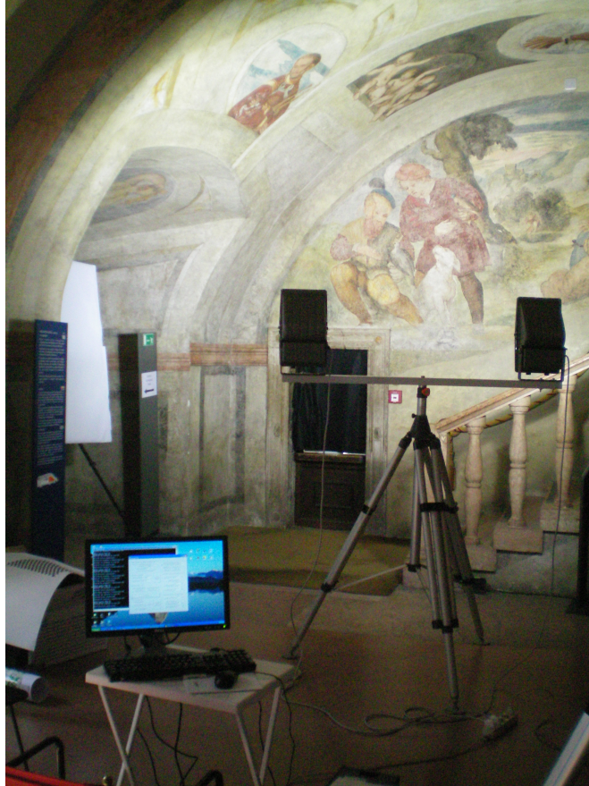
Figure 4.1: Acquisition setup in the Castello del Buonconsiglio, Trento (Italy).
