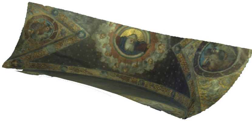
Figure 1.12: Multispectral image of Fig. 1.10 registered on the 3D scan of Fig. 1.11.
