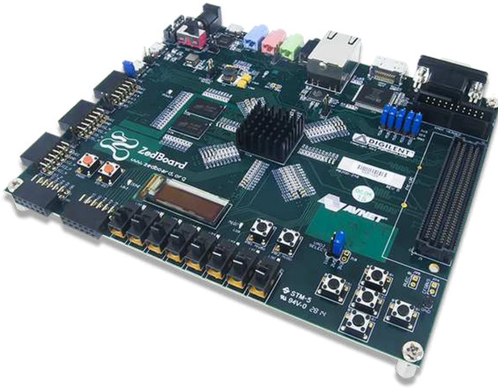
FIGURE 1.1: ZedBoard development kit. Picture by Digilent.
