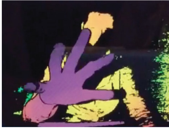
Figure 2.16: Example of pixel-wise independent depth measurements obtained by the Intel RealSense F200 depth camera. The edges of the framed hand are pixel-precise and do not present edge jaggedness typical of spatial multiplexing techniques.
