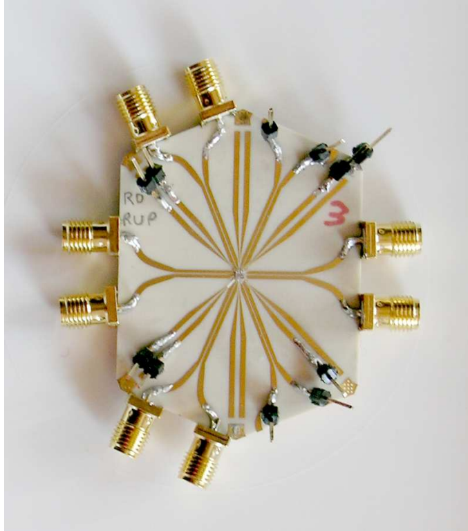
Figure 2.28: CMOS X-band upconverter chip mounted on the test board
