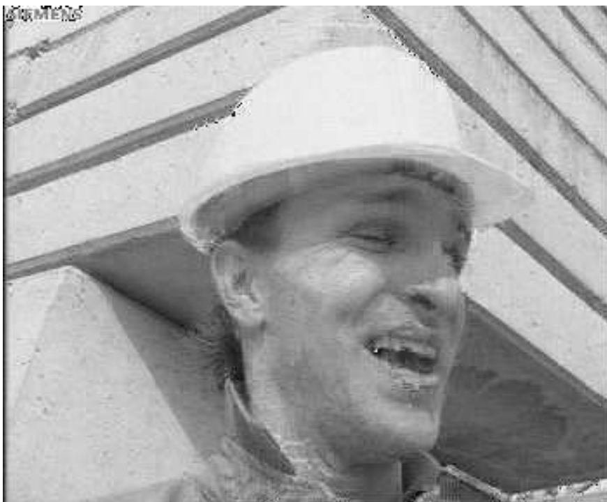
Figure 3.23: Example of video corruption after five transmission errors for MDEZW. The introduced distortion is similar to the artifacts obtained in image compression by truncating the bitplane encoding before all coefficients have been compressed at the resolution necessary for lossless encoding.
