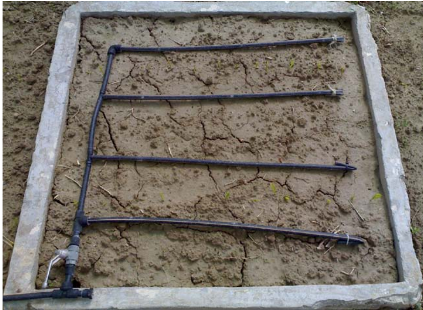
Figure 1.c – particular of a lysimeters and of the irrigation system (by drippers). Picture was taken 2 weeks after sowing.
