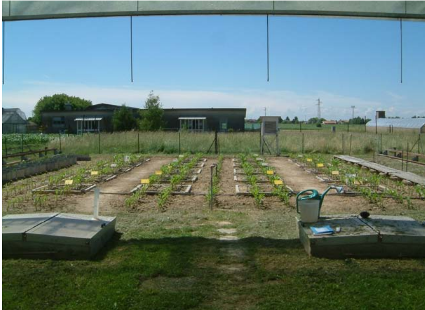
Figure 1.a – Experimental site with 20 lysimeters and 2 under ground sampling chamber. At the top, the automatic sliding roof.
