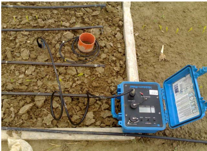
Figure 1.d – TDR (Moisture Point ® , TDR MP 917) and probes (profiling probe Moisture Point ® PRB-F; Moisture Point ® single diode probe SDP) to measure the moisture of soil. In this lysimeter two probes were installed: a 90 cm probe (on the left) and 30 cm probe (on the right).
