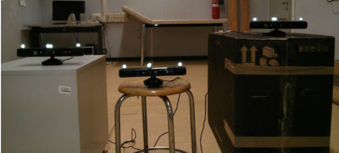
Figure 5.11: One of the test scenarios. Four markers are placed on each kinect in order to recover their locations by means of a motion capture system.
