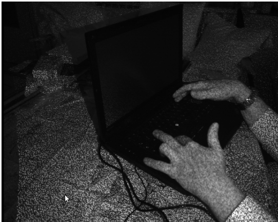
(a) Infrared image acquired by the infrared camera. The projected pattern is clearly visible.
