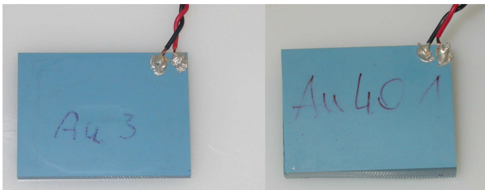
Figure 90 : terminal wires connected by conductive epoxy resin (10-layer left and 40-layer right)
