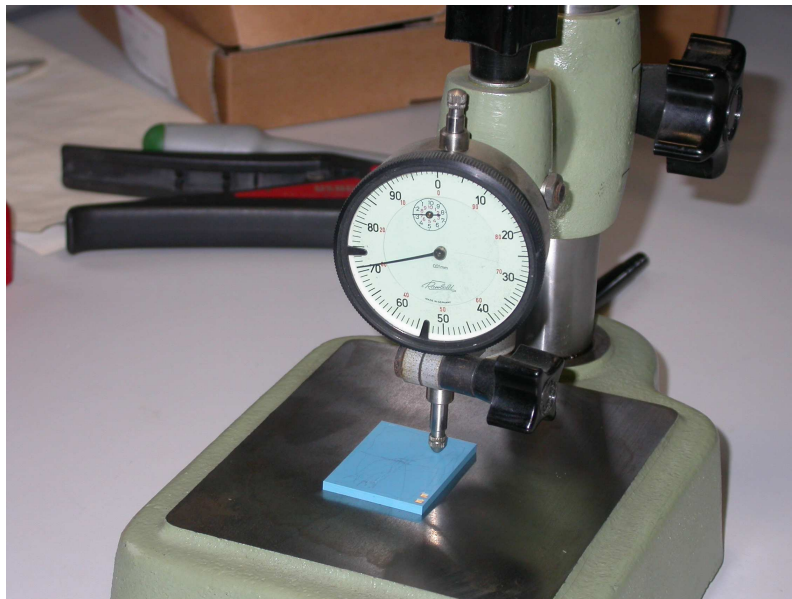
Figure 65: feeler pin used for the planarity test
