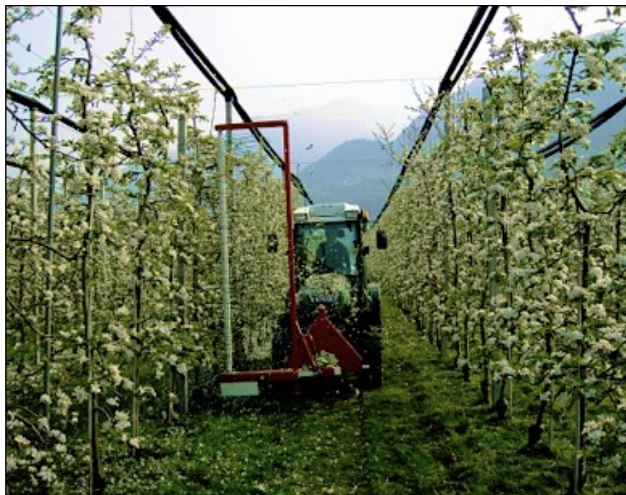
Figure 1 Blossom thinning throughout mechanical device.
