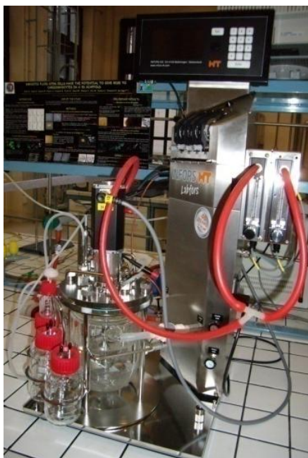
Figure 5. Large scale stirred suspension bioreactor. Provided with water jacket for temperature control, gas inlet and outlet for pH control by CO 2 , stirring system, pumps or on line sampling and feeding. Minimum working volume is 300 ml.
