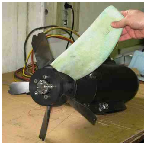
Figure 4.2: Motor bulb with propeller
