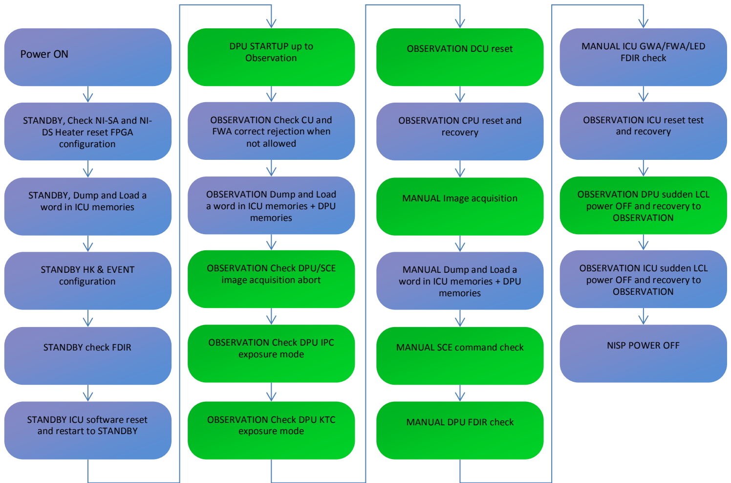
Figure 5.20: FFT Sequence. Violet boxes represents test cases involving the ICU and the NI-OMA simulator, green boxes are for test cases involving ICU and DPU. NISP status is given in each box. Some scripts which include FDIR testing were not included in the NISP AVM delivery in June 2018, they will be part of a second delivery in Fall 2018.
