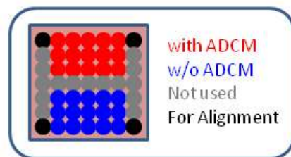
Fig. 193 Apertures layout of the new EG to be installed on NITS for the first Joint Experiments.
