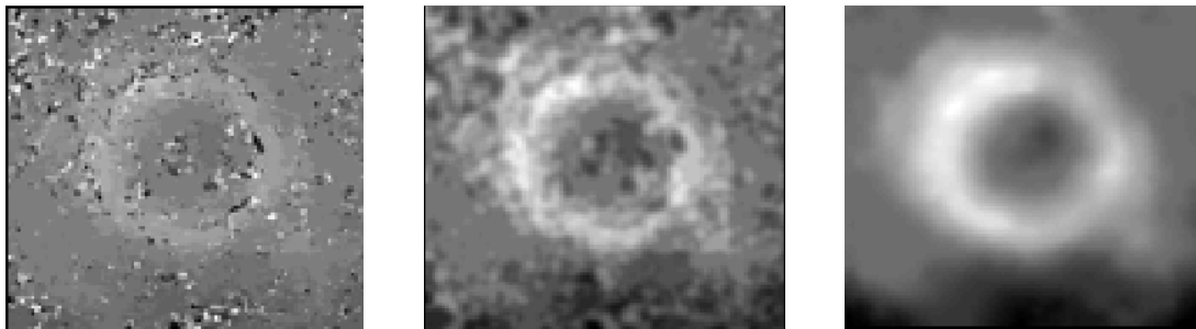
Figure 7 Standard deviation of the differences between the true DTM and the DTM reconstructed by the snake-based algorithm. The theta parameter (see Chapter 3) represents the ratio between the magnitudes of the internal and external forces.
