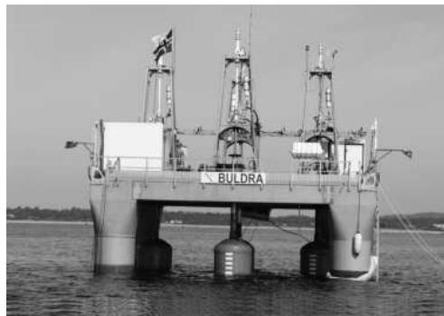
Figure 8.1: Buldra wave energy converter test platform (1:5 model) with hydraulic PTO
