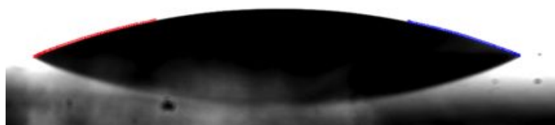
Figure 4.8: Image representing the error fitting procedure used for determining angle contact values in Fig. 4.5d of the manuscript. - Red and blue circles establish chosen zone of drop for performing fitting.
