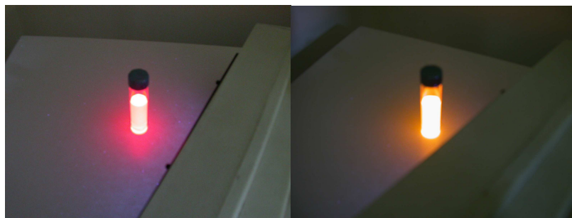
Figure 3.29 Emission from colloidal solution of orange-emitting C2-CSS (left) and yellow emitting C1-CSS (right) under standard UV-lamp illumination (Glass vials are 1 cm in diameter and 6 cm height)
