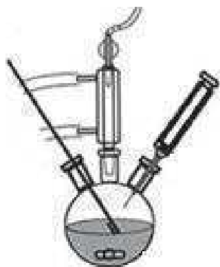
Figure 3.16 Typical experimental set up for “hot injection protocols” for QD synthesis
