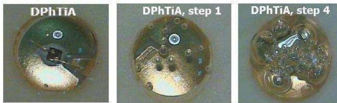
Figure 5.33 DphTi depositions through the syringe dispensing method soon after depositions and at different stages of the curing profile
