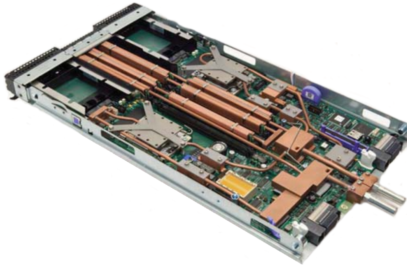
Figure 1.12: Water-cooled IBM BladeCenter HS22 with two high performance micro-channel liquid coolers that remove heat from the microprocessors and various further heat sinks that collect heat from other components, Sridhar et al. (2011) .
