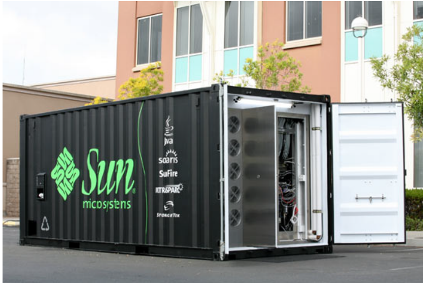
Figure 1.18: The Sun Microsystems Modular Data Center, a portable Data Center built into a standard 20-foot long (6.1 meters) intermodal container.
