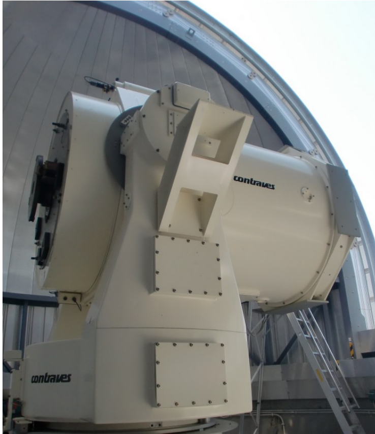
Figure 5.5: Picture of the MLRO telescope system and coudé path.
