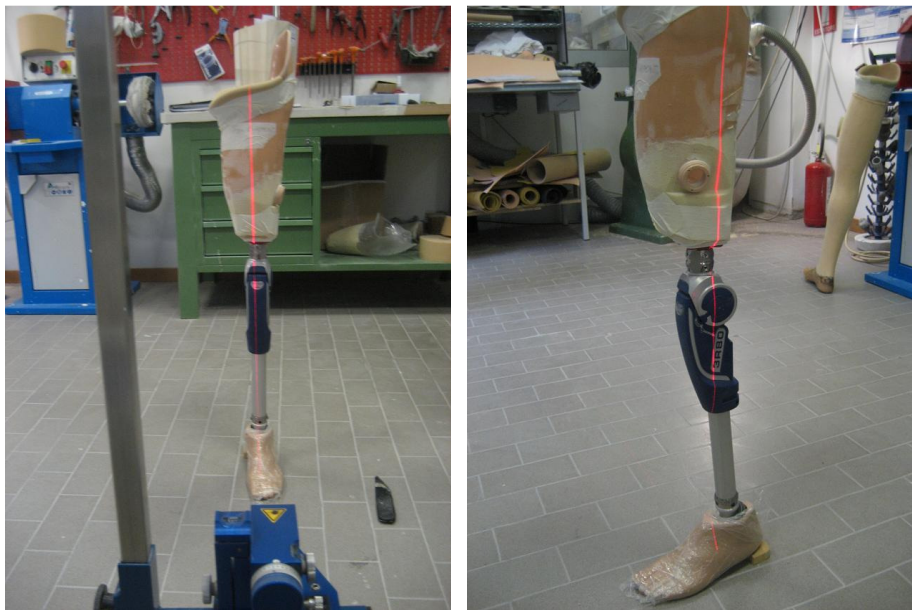
Figure 2.63: Example of static alignment of TF prosthesis with a resin socket, frontal (left) and lateral (right) view.
