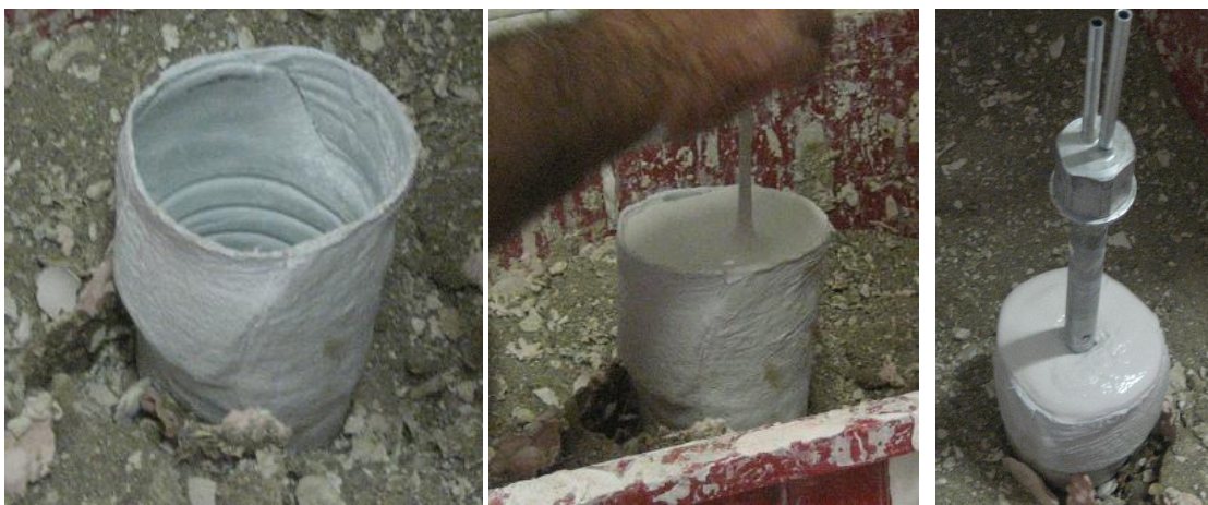
Figure 2.46: Negative cast positioned into the sand bin (left), liquid plaster drained into the cast (centre) and metal tube inserted (right).
