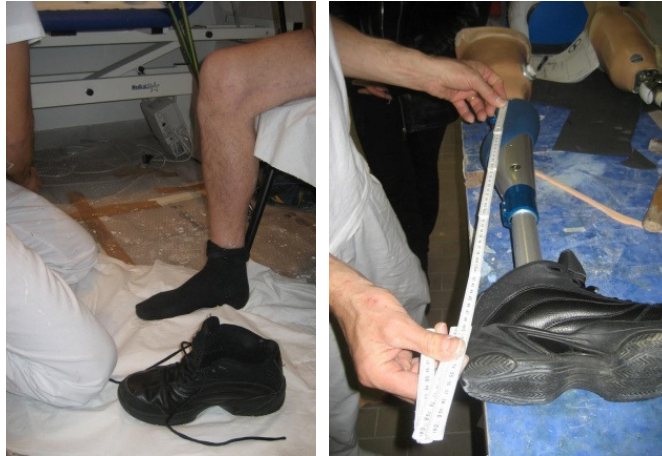
Figure 2.31: Position of the limb to measure the knee height (left) and measurement of the prosthesis knee height for a TF prosthesis (right).
