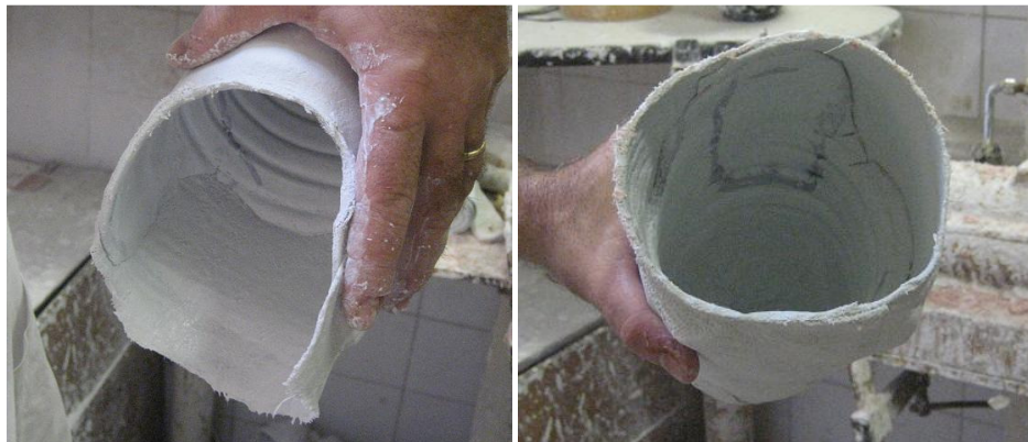
Figure 2.44: Plaster bandages added to the upper edge of a TT cast (left) and final result (right).
