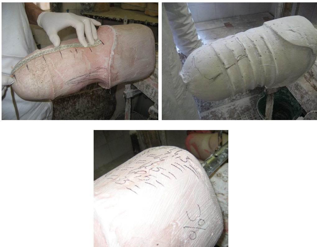
Figure 2.47: Reference circumferences reported on a TF positive cast (upper left) and on a TT cast (upper right), and an example of calculation of percentage range of downsizing (below).
