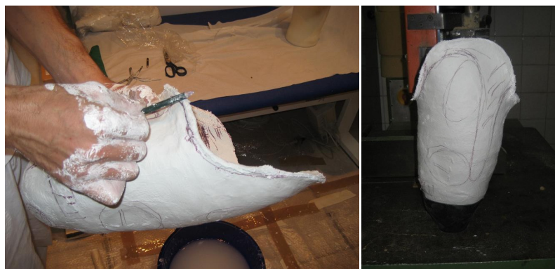
Figure 2.41: Alignment of a TF negative cast (left) and position on the rubber base (right).
