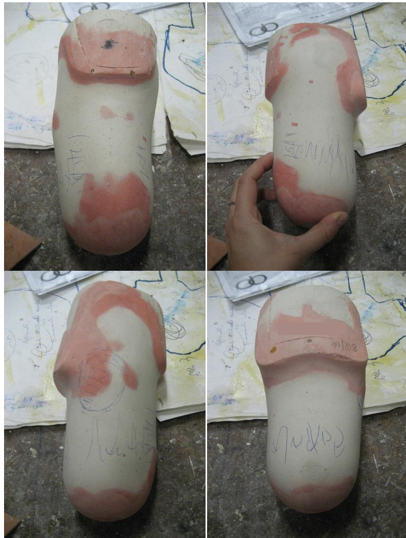
Figure 2.59: Positive TT stump with drawn the areas , which have to be modified, from the left to the right, from up to down, we have respectively: frontal, internal lateral, internal external and back view.
