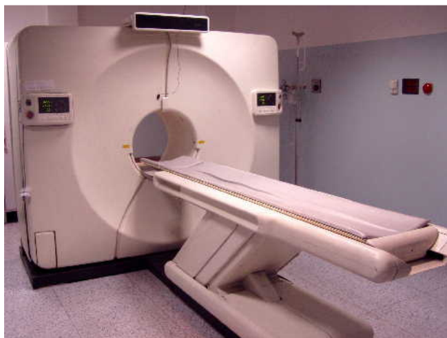
Figure 1.18: Example of PET tomograph.
