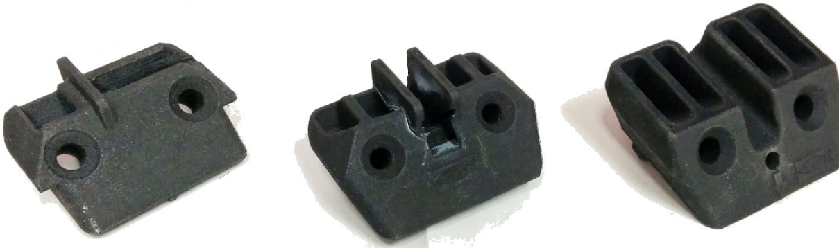
Fig. 2.11 – Prototypes realized by stereolithography.
