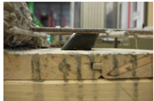
Fig. 2.16 – Detail of Connector and screw installation onto the timber beam.
