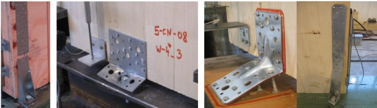
Fig. 3.3 – Example of brittle or “less ductile” failures occurred on experimental tests ([3.21];[3.24]) and lateral yielding of an hold-down due to coupling effects [3.9].
