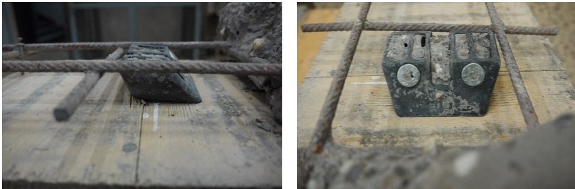
Fig. 2.22 – Investigation of connection after failure: (a) screw withdrawal with partial rotation of the plastic element; no critical failure observed in the thermoplastic connector.
