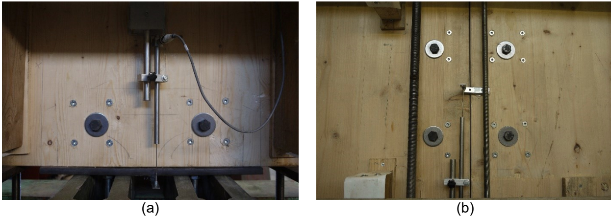
Fig. 3.33 – Position of LVDTs to assess displacements of each bracket for tension tests (a) and shear test (b).
