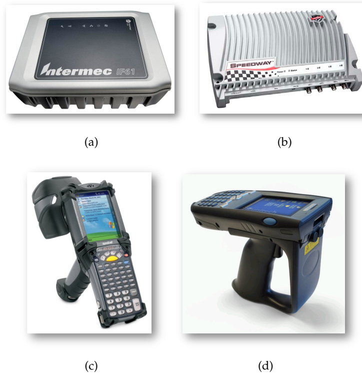
Figure 1.6: Examples of readers: (a), (b) fixed readers; (c), (d) handheld readers.
