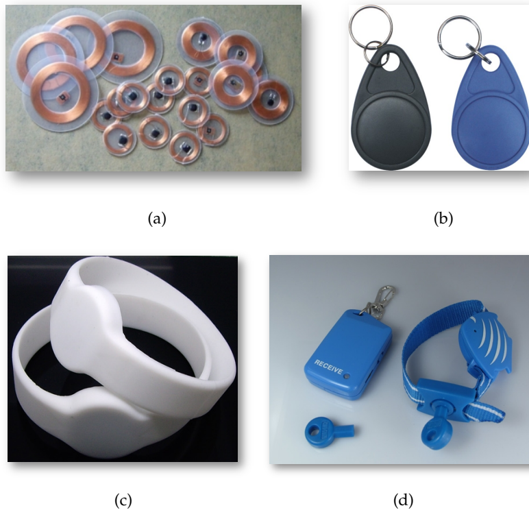
Figure 1.5: Examples of tag enclosures: (a): LF and HF tags with coil shaped antennas; (b): tags are inserted inside a key; passive (c) and active (d) wristband for local monitoring applications ( i.e. for children).
