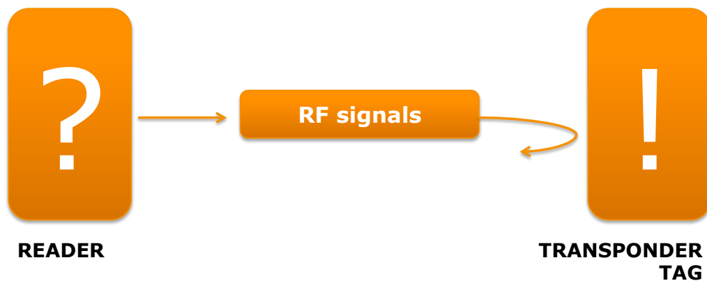
Figure 1.7: The simplest model for an RFID system: the device marked as “interrogator” (or “reader”) emits a signal to communicate with a second device, the “transponder” (or “tag”). The question mark identifies the interrogating device because its fundamental function is basically to broadcast a request for identification. On the other side, the basic function of a tag is to answer the interrogation, identifying itself. The communication protocol is based on radio frequency electromagnetic signals.
