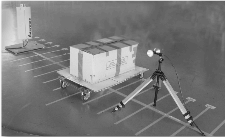
Figure 4.1: Picture of the testbed adopted. The image shows the target of identification process, and a measurement antenna used to detect power levels.
