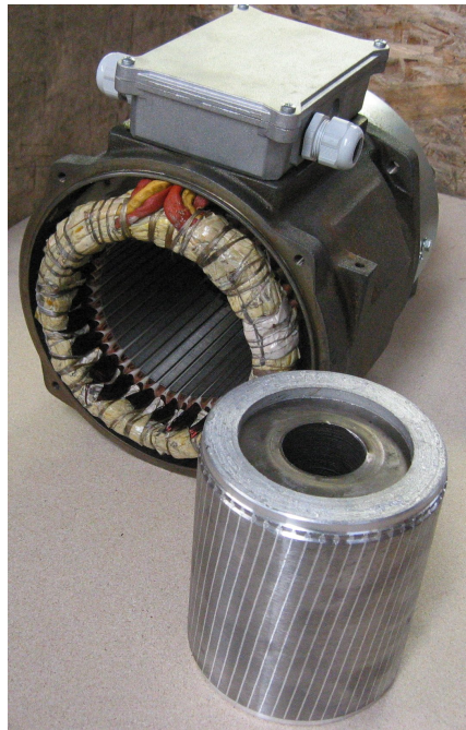
Figure 2.2: Rotor and stator of the realized motor for the elevator system. Courtesy of EME spa.
