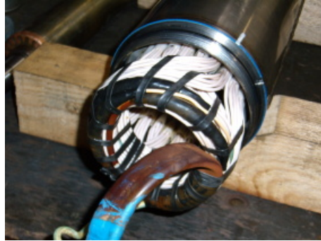
Figure 3.4: The end winding of the submerged pump IM. Courtesy of Lowara.
