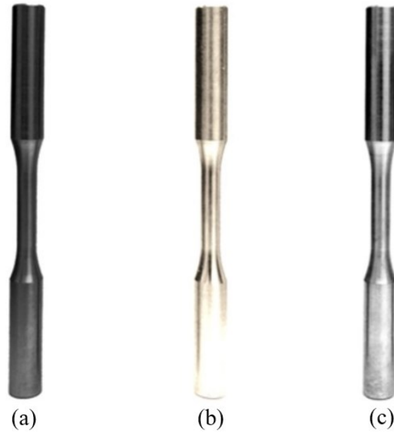
Figure 32: Specimens sets (a) Set 1: as received, (b) Set 2: zinc coated Fe/Zn5/a, (c) Set 3: nickel coated Fe/Cu1/Ni5s
