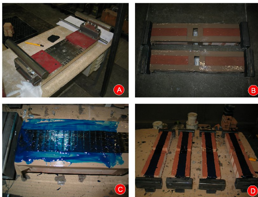
Figure 6.11: Images taken during the specimens preparation: device for flexural tests (A), two samples before the FRP application (B), bonding of fibres (C) and specimens ready for testing (D)
