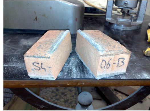
(b) Failure of a brick
