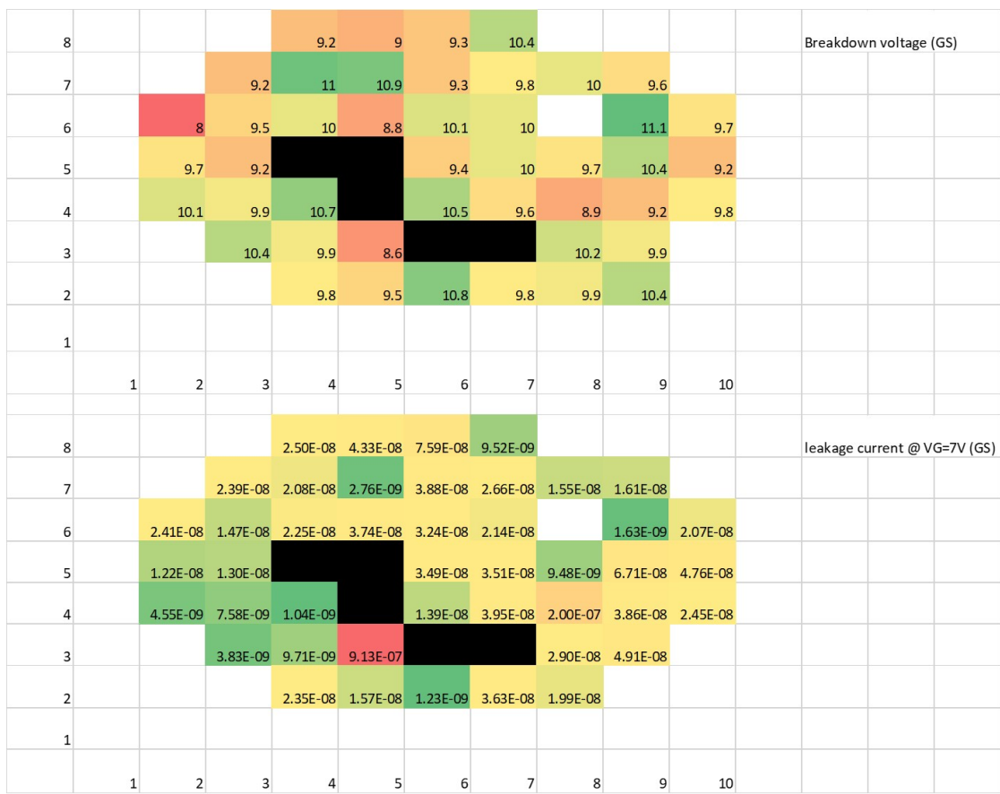
Figure 4.13 – The spatial map of leakage (at 7 V) breakdown voltage. The leakage current and breakdown voltage strongly depends on the cell position and on the device topology.
