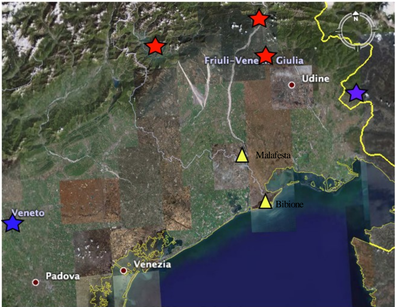
Fig.10 Earthquakes recorded. Yellows Triangle are the installed stations. In red star earthquakes coming from dangerous seismogenic zones, in blue star earthquakes coming from lateral directions.
