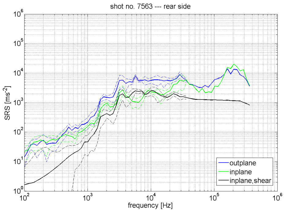
Fig. 6-33. Type of waves for dp=1mm (below BL). Rear side
