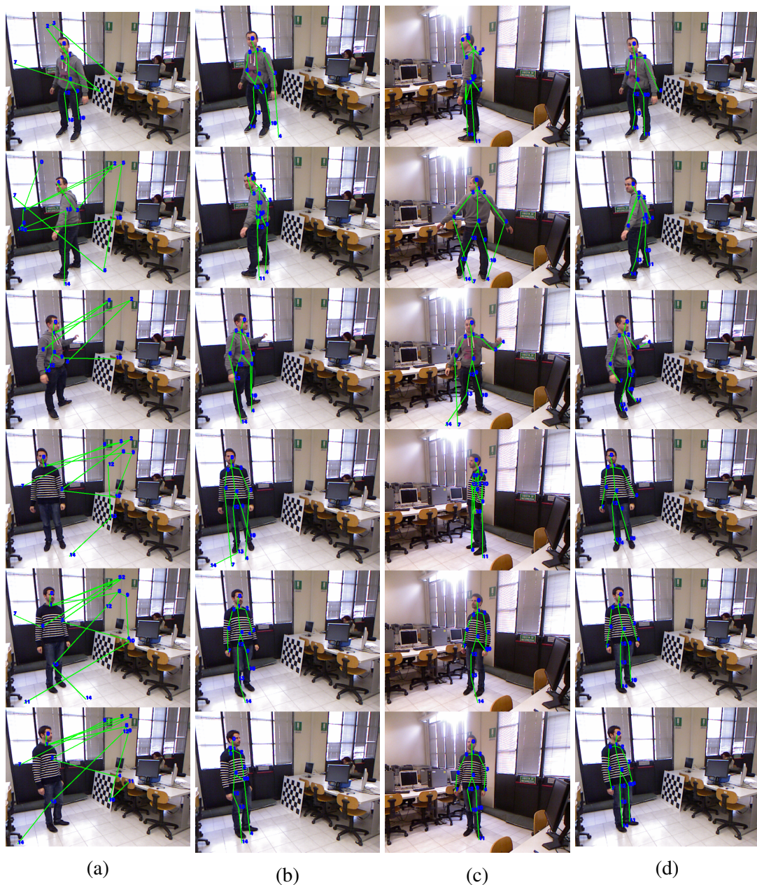
Figure 3.5: Some sample frames of the dataset we used for testing the proposed approach. Each row represents a frame. The different columns represent: a) [12] on the C_0 stream; b) ours with PD and JT on the C_0 stream; c) ours with PD and JT on the C_1 stream; d) our multi-view approach re-projected on the C_0 camera.
