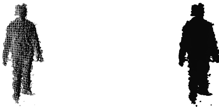
Figure 3.4: On the left, the resultant point cloud re-projection to the image plane of the reference camera. On the right, the re-projection after the hole-filling procedure.
