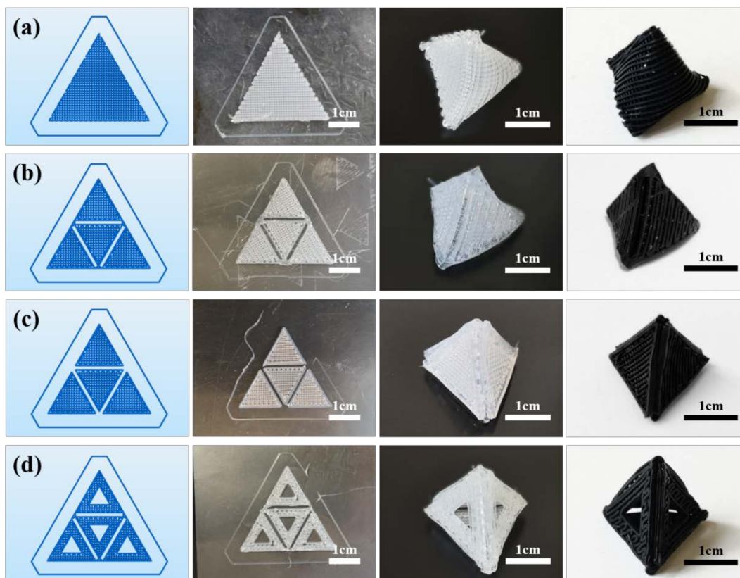
Fig. 2.7 Illustration of different processing possibilities to fabricate a tetrahedron structure: (a) folding and binding of a single sheet; (b) folding and binding of a single sheet containing different structures, linked at the edges; (c) assembling and binding of separate parts; (d) folding and binding of a single sheet containing different structures with additional porosity, linked at the edges. A silicone filament was used to bind the different parts, in all examples.
